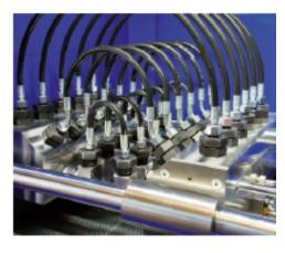
Pressure impulse test and hydrostatic testing in accordance with the common Standards, including flexing and half-omega Due to freely programmable pressure curves and axis movements, tests can be realized even beyond the Standards.
